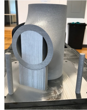
Tee Built using PBF 4" Diameter x 8" Tall \cong 50 lbs. (Rolls-Royce)
