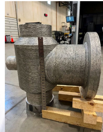
Valve Built Using Gas Metal Arc DED 8" Valve \cong 1000 lbs. (EPRI/ Lincoln Electric)
