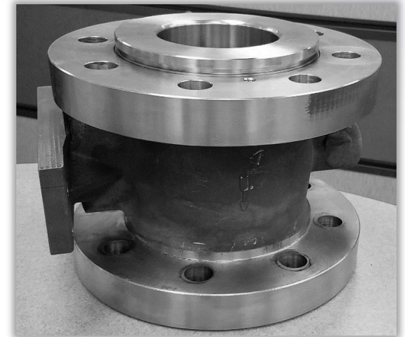
Valve Body using PBF AM Courtesy of Emerson
